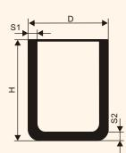
Non-glazed crucibles are used for casting of non-ferrous metals and their alloys with temperature not more than 1600°C. They are remarkable for their increased thermal insulating properties. Glazed type is possible if requested by consumer.
