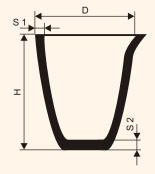
Non-glazed crucibles are intended for melting of precious metals with melting temperature up to 1600°C in the induction and muffle furnaces.
