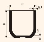
Glazed crucibles are intended for melting and distribution of non-ferrous metals and alloys with melting temperature up to 1600°C.
